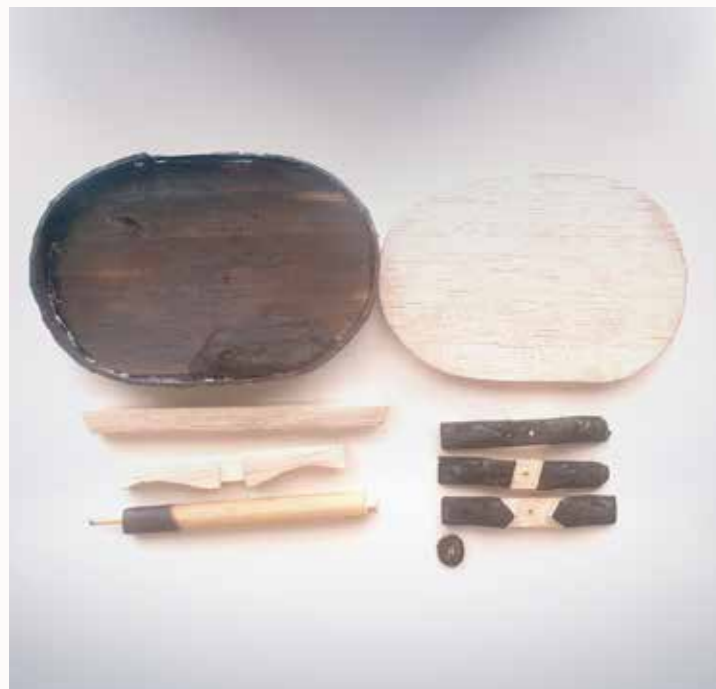
Physical prototype at 1:5 scale using balsa wood and timber dowels.
